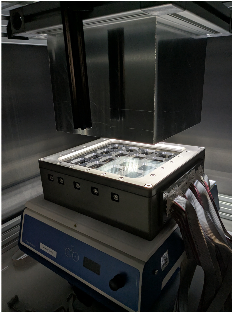
Figure 3.2: Environment chamber mounted on a hotplate under the LED array with mirrored walls for improved uniformity.
