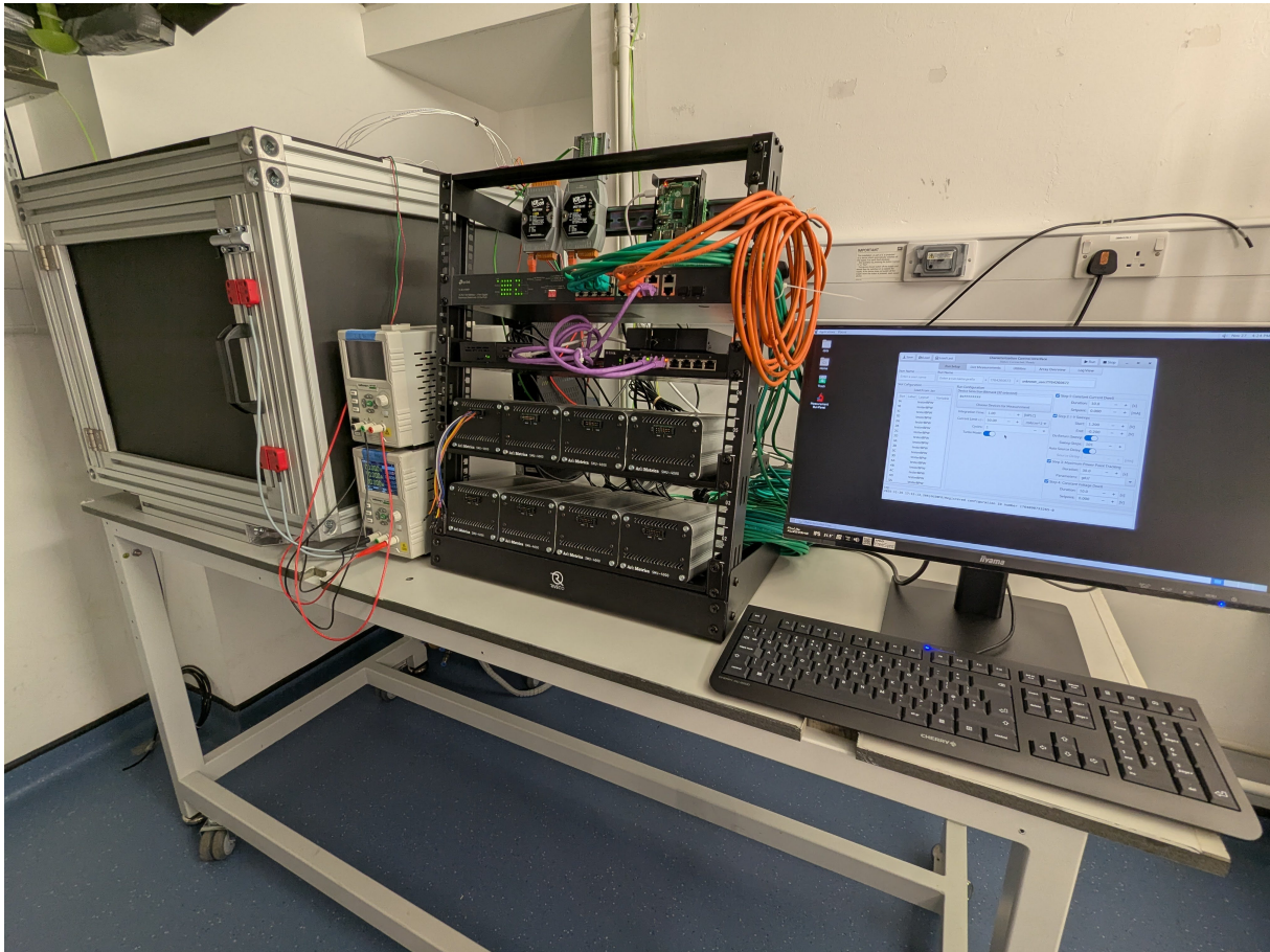
Figure 4.3: System photograph showing enclosed lightsource, 32 rack mounted SMU channels, and the control computer.
